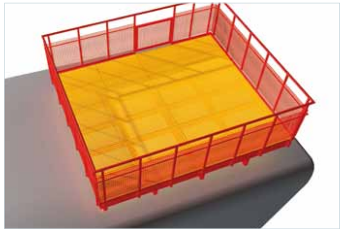
Possible basic structure of a helihoist
