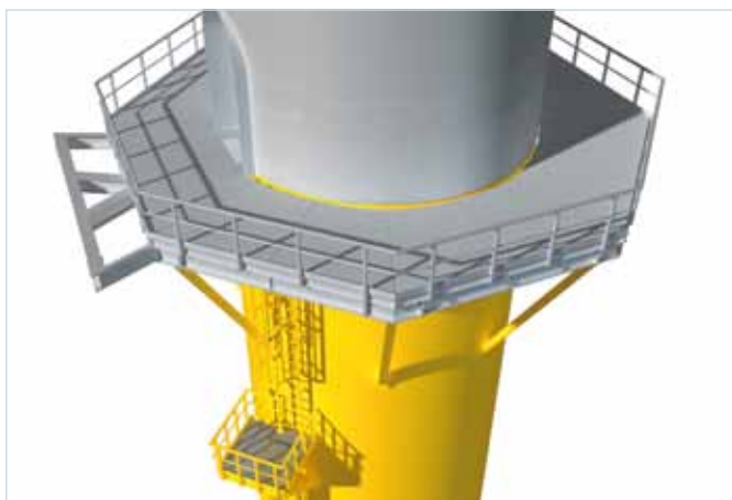
External platform at the monopile
